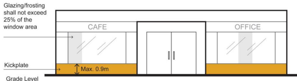
Figure 28. Building Façade Regulations
